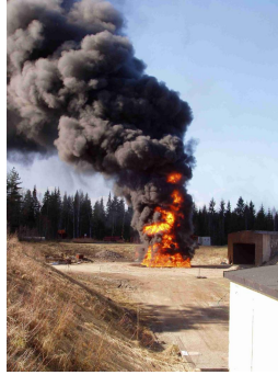
Fast Cook Off test with liquid hydrocarbon fuel
