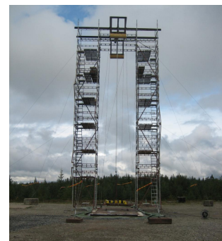
12 m drop tower for large test items
