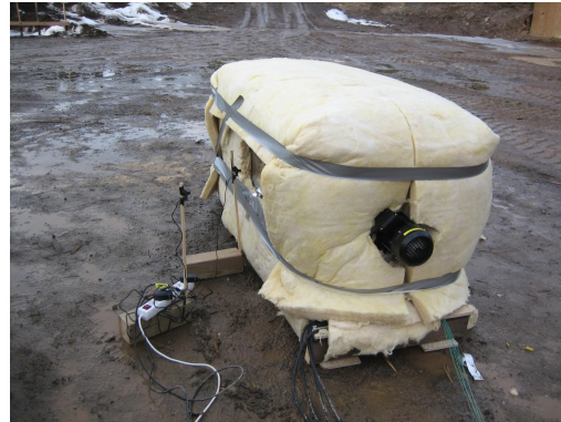
Slow Cook Off oven with extra insulation and video cameras
